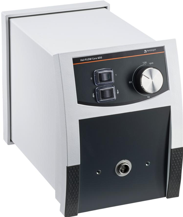
This pump of the Hei-Flow Core series is particularly suitable when high volumes need to be transported easily. A flow rate of 4.0 - 4,151 ml / min can be set for this purpose. This model is designed for the use of single-channel pump heads.
