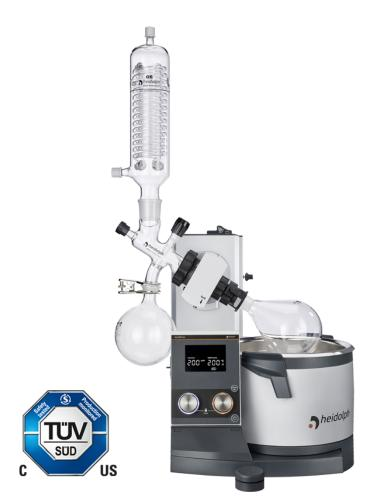
An operating concept that is focused on the essentials: clear and with access to the basic parameters rotation speed and heating bath temperature at any time.
