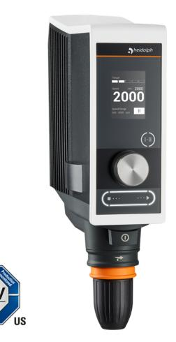
With Hei-TORQUE Expert 400 you can optimally stir viscosities up to 250,000 mPas or volumes up to 100 liters ( $H_2O$ ). Thanks to its 2-gear stage design, it stirs particularly powerfully in the speed range up to 400 rpm and is therefore particularly suitable for applications with highly viscous media that require mixing in the lower speed range. However, operation at speeds of up to 2,000 rpm is also possible in the second speed.
