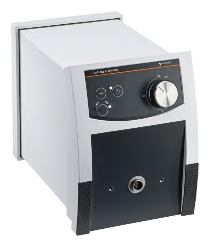
This model has a flow rate of 2.0-4,056 ml/min and is designed for operation with single-channel pump heads. The analog interface makes it possible that all functions can be controlled externally. A control accuracy of  $\pm 3.5\%$  and a conveyor speed of 24 to 600 rpm provide optimum process conditions. In addition, sensitive media can be protected from influence by using the optional foot switch.
