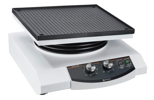
Containers are safely fixed on the anti-slip rubber mat even at high speeds. The speed is variably adjustable between 2 and 50 rpm. The shaker can be operated in continuous operation or with a timer (max. 120 minutes).
