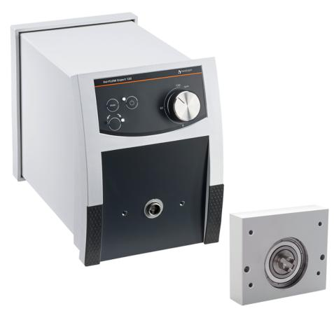
The pump drive of the model 120 of the Hei-FLOW Expert series can be operated with either single-channel or multi-channel pump heads. The flow rates with single-channel pump heads are in the range of 0.38 - 813 ml/min; with multi-channel pump heads from 0.005 - 329 ml/min.
