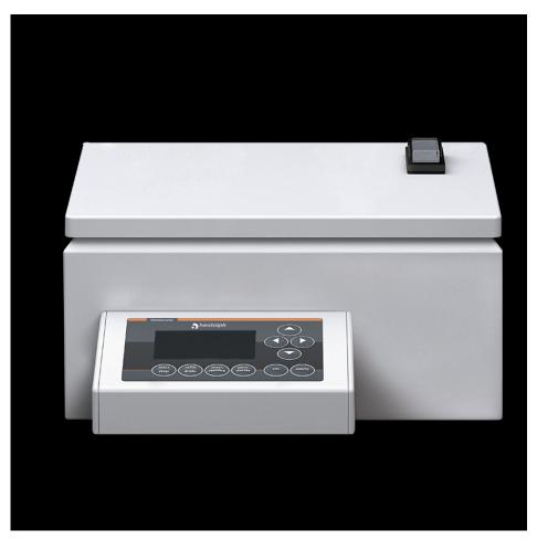
Using the control panel on the control box of the Hei-VOLUME Distimatic module, you can enter the parameters for the sensor or time-controlled filling of the rotary flask, as well as program the emptying time of the coated collector vessel (approx. 700 ml) using the chemical membrane pump. The control box can be mounted directly on any Hei-VAP Industrial large-scale rotary evaporator or on a nearby wall using the supplied bracket with hose guide.
