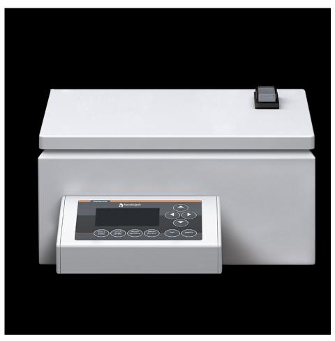
Using the control panel on the control box of the Hei-VOLUME Distimatic module, you can enter the parameters for the sensor or time-controlled filling of the rotary flask, as well as program the emptying time of the coated collector vessel (approx. 400 ml) using the chemical membrane pump. The control box can be mounted on a nearby wall using the supplied bracket with hose quide.
