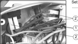
Set of fuses Rot.-Valve Contr./Rotavac 20
