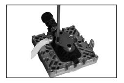
Loosen the clamping brackets on the valve heads.
