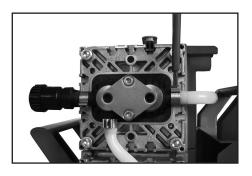
Detach the coupling of the connection tube to the other side of the pump as well as the hose connection to the inlet/outlet of the vacuum system at the valve head.
