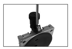
Loosen connection fastener slightly.
