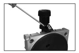
Open the hinged cover of the connection fastener with a slotted screwdriver.
