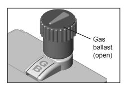
To reduce condensation in the pump, do not pump vapor before the pump has reached its operating temperature. Open the gas ballast valve when pumping condensable vapors.
