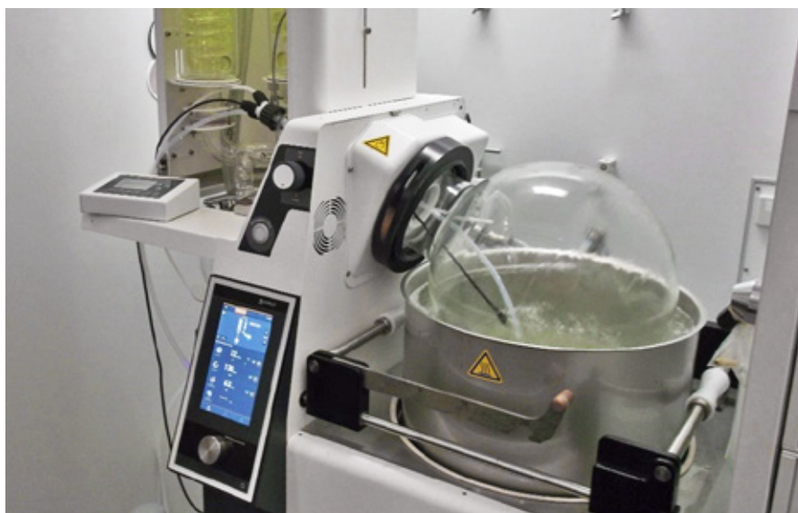
Fig. 1: Hei-VAP Industrial with Distimatic test setup
